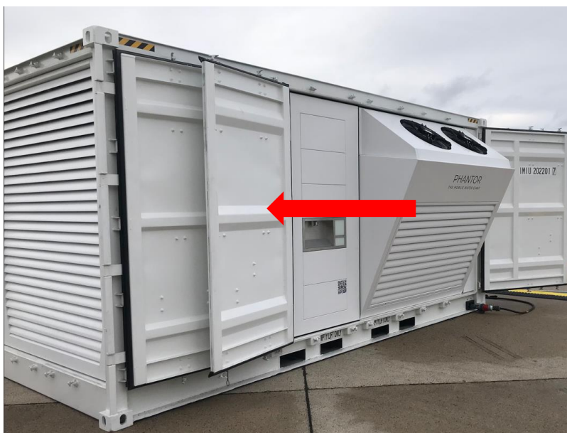
Figure 10: Container door in front of water kiosk
