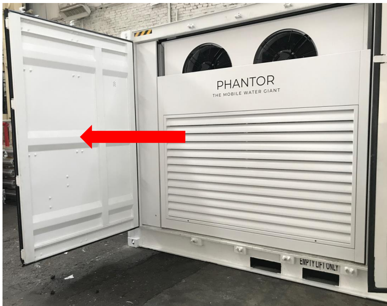
Figure 9: Opening the two longitudinal container doors in front of the condensers
