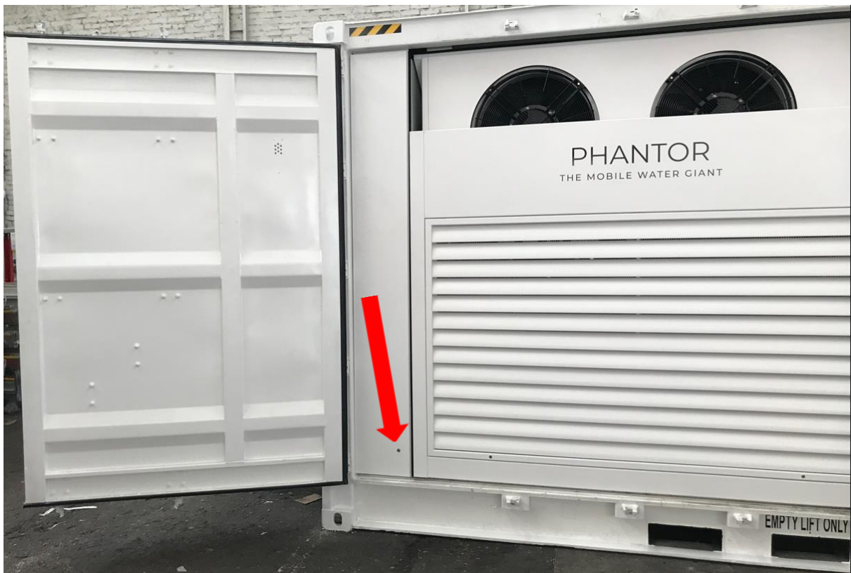
Figure 11: Key switch (arrow) for extending the condenser
