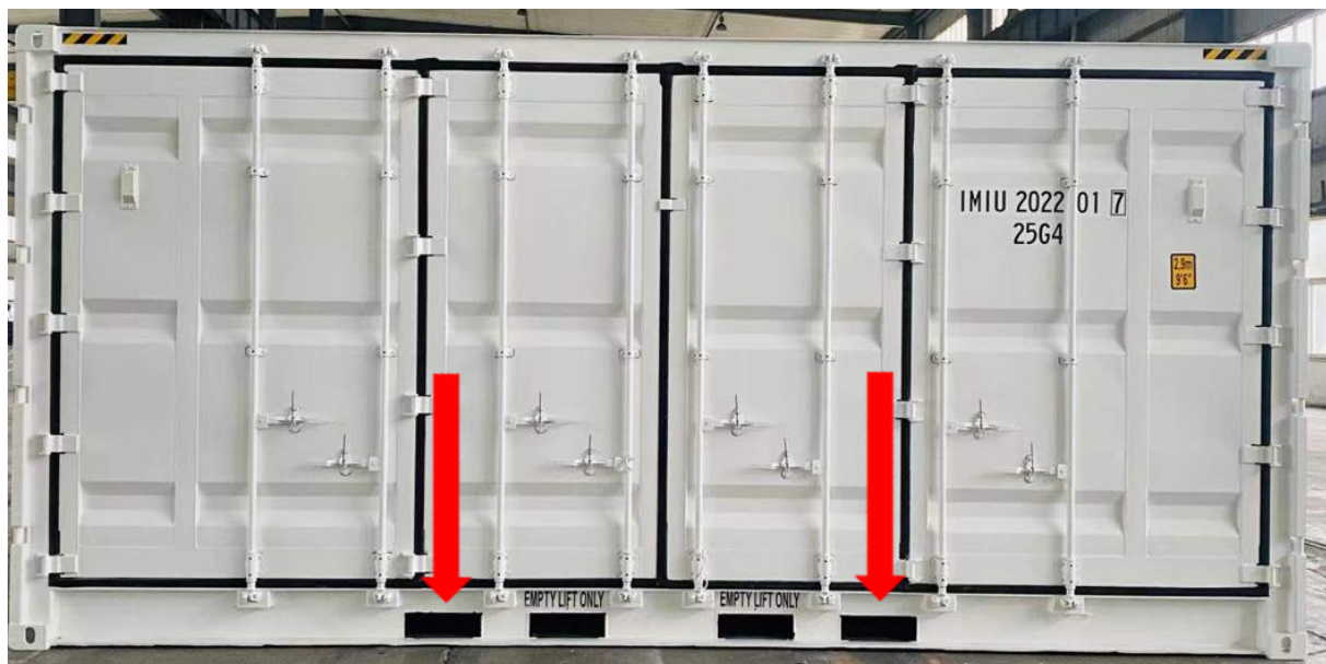
Figure 24: Lifting openings for lifting by forklift truck
